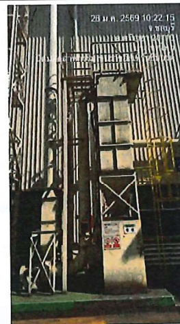
Dust Collector G.8 Forging 4
